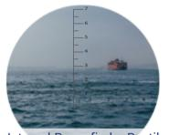
Internal Rangefinder Rectile
